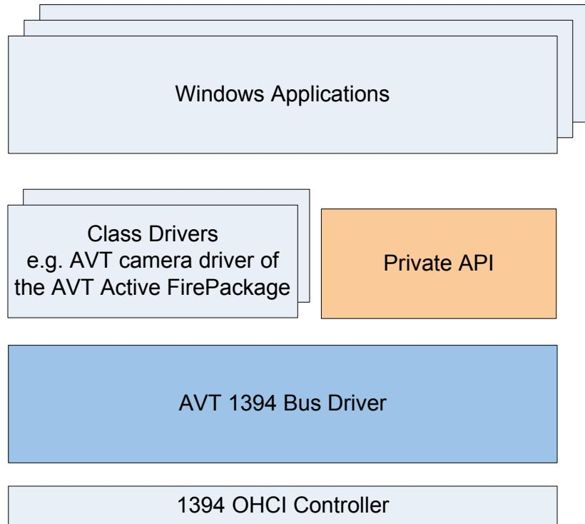
Figure 18: Architecture of **AVT 1394 Bus Driver**
